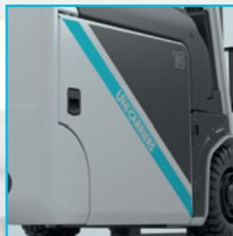
Change batteries easily with a pallet truck (rollout exchange optional).
