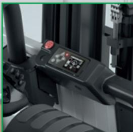
Onboard pre-operation checklist and overload alarm. An interactive truck with a safe operation indicator.
